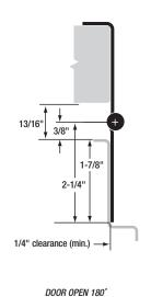
MATERIAL: 14 gauge 304 stainless steel with 3/16" diameter 304 stainless pin. Long-life nylon medical bearings.
