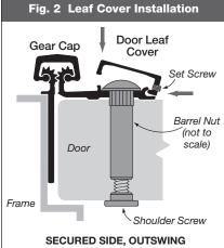
**NOTE:** For inswing applications, reverse position of barrel nut and shoulder screw so that the shoulder screw is on the secured side of the door.
