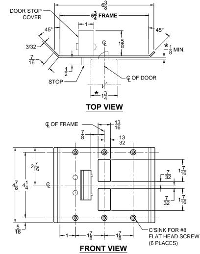
STOP IS SPRING LOADED MAKING PART NON-HANDED BUT INSTALLATION IS STILL HANDED
