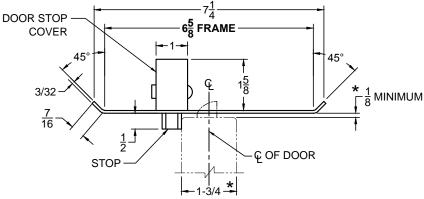
STOP IS SPRING LOADED MAKING PART NON-HANDED BUT INSTALLATION IS STILL HANDED
