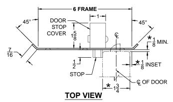
STOP IS SPRING LOADED MAKING PART NON-HANDED BUT INSTALLATION IS STILL HANDED
