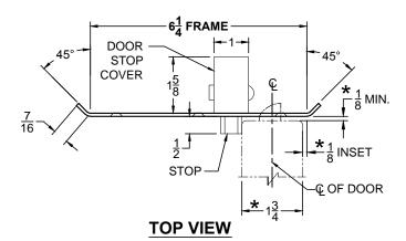
STOP IS SPRING LOADED MAKING PART NON-HANDED BUT INSTALLATION IS STILL HANDED
