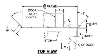
STOP IS SPRING LOADED MAKING PART NON-HANDED BUT INSTALLATION IS STILL HANDED
