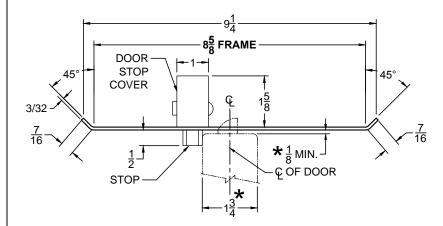
STOP IS SPRING LOADED MAKING PART NON-HANDED BUT INSTALLATION IS STILL HANDED
