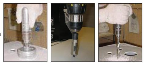
Using a drill with a positive rake angle and thin points or split points can help reduce cutting pressure and thus delamination at both entrance and exit. Feed rates must also be constant and may even be reduced upon exiting from a hole to reduce flexing of the part when the drill exits. Using a solid back surface to support the part when drilling can also aid in reducing delamination and chipping.
