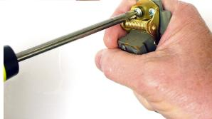
Step 4: Inspect the long handle bracket to make sure it is straight and flat. Sometimes these brackets are bent as a crude form of installation adjustment. This is <u>not</u> recommended. The handle bracket must be flat and straight to work with the 2740-117 retrofit kit. Flatten and/or straighten as necessary.
