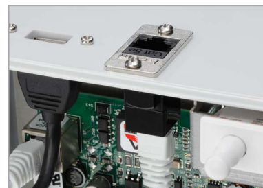
PIM400-1501 has RJ-45 and USB external connectors to make installation easy.
