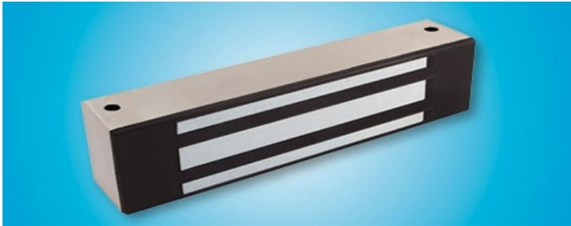
Magnetic lock providing 600lbs of holding force with fully sealed electronics protected from water and dust, surface mounted with minimal tools, mounted using steel machine screws into finishing nuts, ten feet [3.05m] of jacketed, stranded conductor, operates with 12 or 24V DC power.
