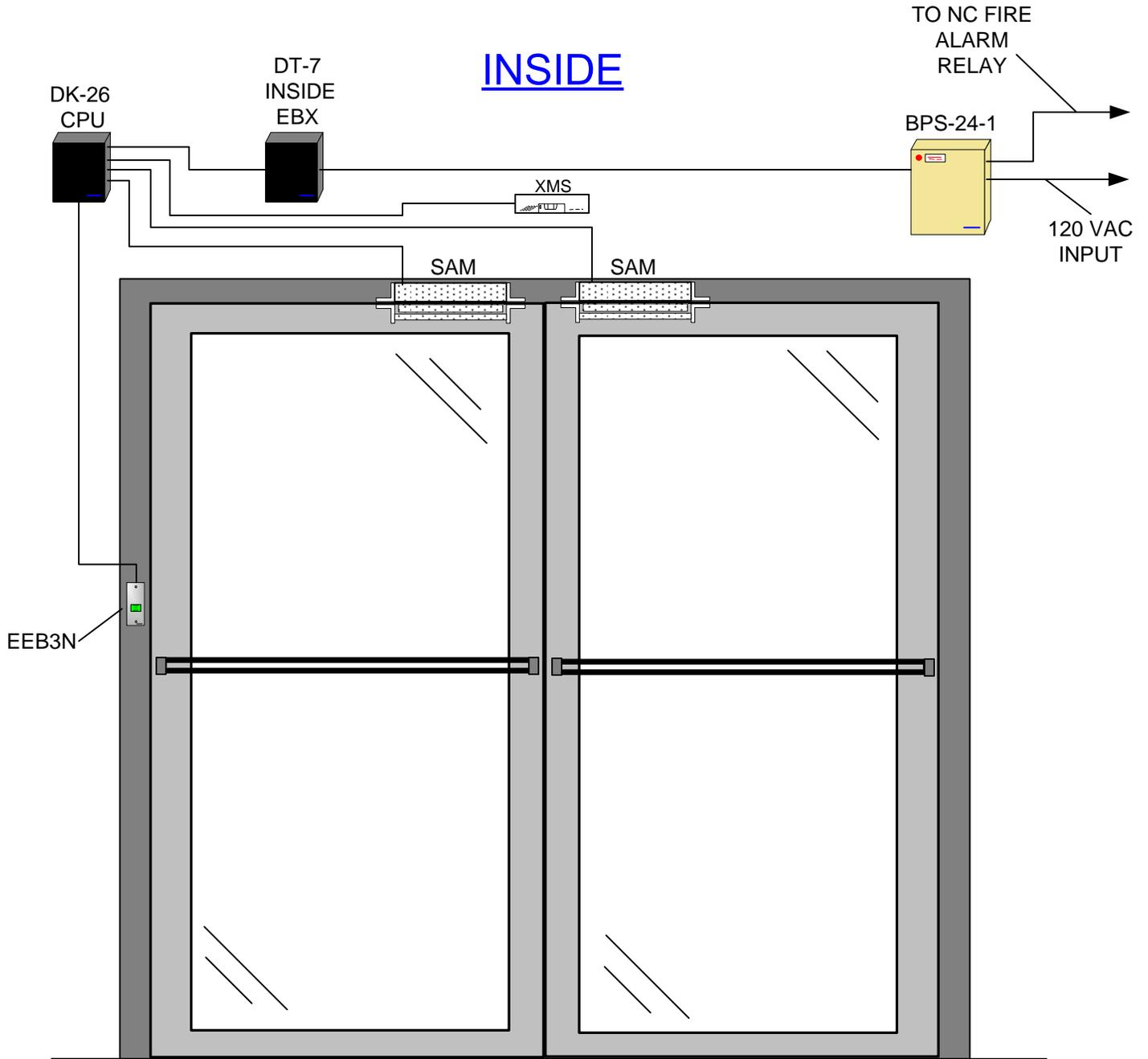
COMMENTS: MOST DEVICES COME WITH WIRE LEADS IN DIFFERENT LENGTHS DEPENDING ON WHAT MODEL IT IS. IF LONGER WIRE RUNS ARE REQUIRED 18G STRANDED WIRE IS FINE FOR SHORTER WIRE RUNS ON A 12 V SYSTEM. 22G WIRE IS ACCEPTABLE FOR SHORTER WIRE RUNS ON A 24 V SYSTEM. FOR SPECIFIC WIRE GAUGE QUESTIONS ON LONGER RUNS OR SYSTEMS PLEASE CALL OUR TECH SUPPORT LINE AT 1-800-MAGLOCK OR 1-800-624-5625.
