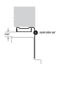
**MATERIAL:** 14 gauge 304 stainless steel barrel with 3/16" diameter 304 stainless pin. Long-life nylon medical bearings.
