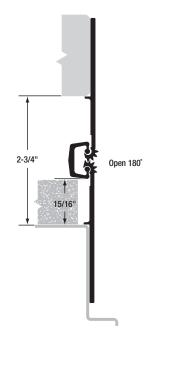
**MATERIAL:** Extruded 6063 T6 aluminum alloy with self-lubricating polyester thrust bearings.
