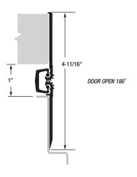
**MATERIAL:** Extruded 6063 T6 aluminum alloy with self-lubricating polyester thrust bearings.
