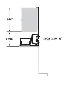
**MATERIAL:** Extruded 6063 T6 aluminum alloy with self-lubricating polyester thrust bearings.
