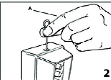
The combination for the outside and inside locks must be changed independently. Follow the same procedure for the outside and inside.
