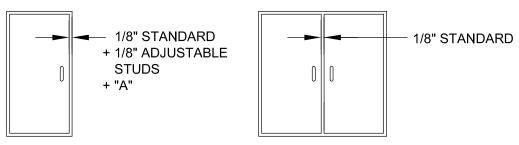
Proper door reinforcement is required for adjustable feature.
