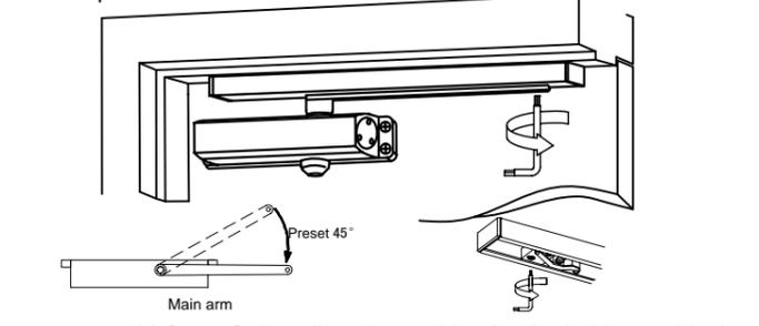
2. For Hold Open Only, adjust the position for the hold open block in the track in order to adjust the hold open angle. If you don't want the hold open function, please don't use the hold open lock.
