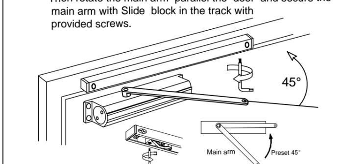
2. For Hold Open Only, adjust the position for the hold open block in the track in order to adjust the hold open angle. If you don't want the hold open function, please don't use the hold open lock.
