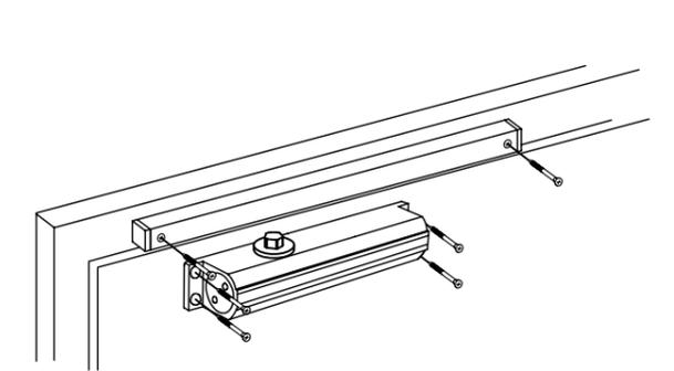
**4** 1. Put the main arm on the upper shaft make sure the included angle is 45° between the main arm and door (preset load). Then rotate the main arm parallel the door and secure the main arm with Slide block in the track with provided screws.
