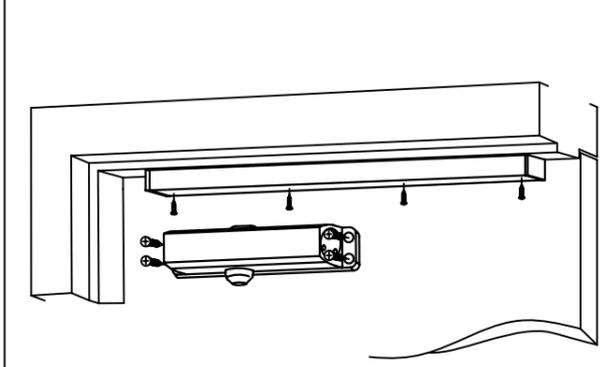
**4** 1. Put the main arm on the upper shaft make sure the included angle is 45° between the main arm and door (preset load). Then rotate the main arm parallel the door and secure the main arm with Slide block in the track with provided screws.
