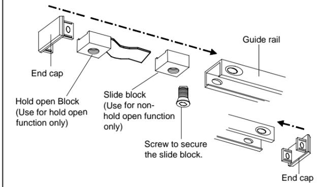
**3** Install the door closer and track according to the drawing.
