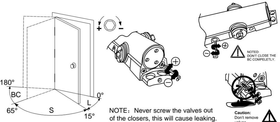
NOTE: Never screw the valves out of the closers, this will cause leaking.
