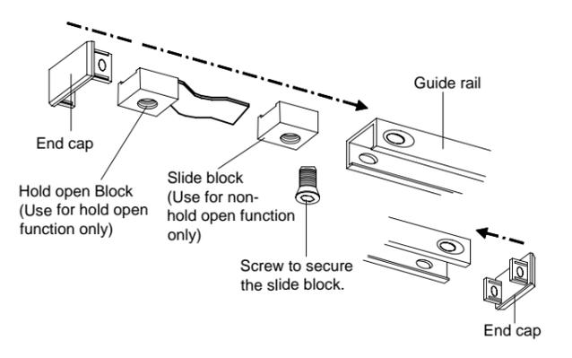
**3** Install the door closer and track according to the drawing.
