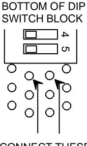
CONNECT THESE TWO PADS BY WIRE JUMPER
