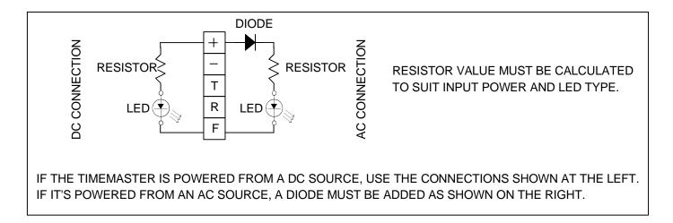
When the time is set to zero in the cyclic mode, the flash out can be employed as an LED flasher to annunciate some condition on a panel (see section 6.5). The F terminal can only operate a resistive load of less than 60 mA or the board will be damaged. It can not operate any incandescent lamp.
