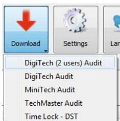
If you select TechMaster Audit a new window will open where you can select which events (lock 1, lock 2, lock 3, lock 4, lock 5 or keypad) and the number of events to download (maximum 6000 events from the lock and maximum 250 events from the keypad).
