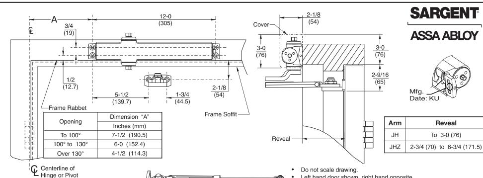
NOTE: These installation instructions to be used for product manufactured on or after Nov. 1, 2013. Date Code: KU Shipped with arm as shown.
