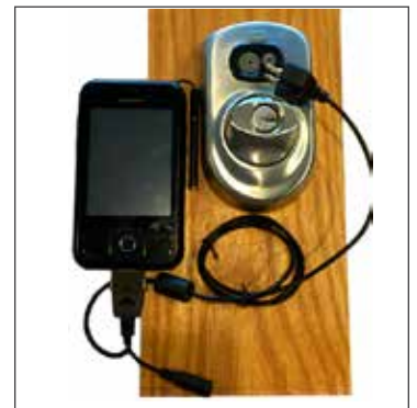
Serial Communication with 2PIN Serial Cable (BM-170)
