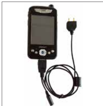
Serial Communication with 2PIN Serial Cable (BM-150)
