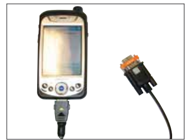
Serial Communication with Null Modem (PIMWA-CV) (BM-150)
