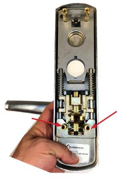
2. REMOVE MOUNTING PLATE & DISCARD. LINE UP REE BRACKETING WITH MOUNTING POST HOLES.
