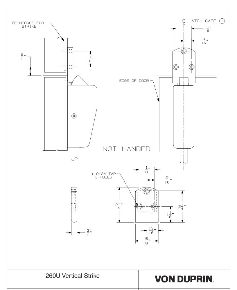
NOTES: Latch case mounting holes to be prepared at installation on door
