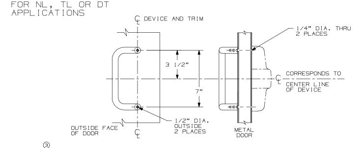
DEVICE APPLICATION SCHEDULE 98/99 SERIES RIM (DT OR NL) 98/99 SERIES SURFACE VERTICAL (DT, NL OR TL) 98/99 SERIES MORTISE (DT OR NL) 98/99 SERIES CONCEALED VERTICAL (DT, NL OR TL)
