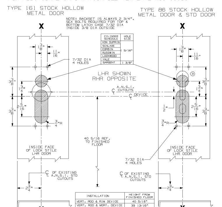
VON DUPRIN CUTOUTS ARE LOCATED FROM A.N.S.I. CUTOUTS SEE A.N.S.I. SPECIFICATION NO. A115 FOR THE SIZE AND LOCATION OF THESE CUTOUTS.
