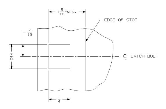
REINFORCED HOLLOW METAL AND ALUMINUM FRAME PREPARATION
