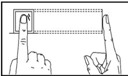
**Make finger center pressed on the sensor window.**
