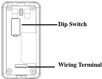
**Dip Switch:** 1-4 switches are used to set the RS485 communication address (device ID). Number 5 switch is idle. And the number 6 switch is used to set the terminal
