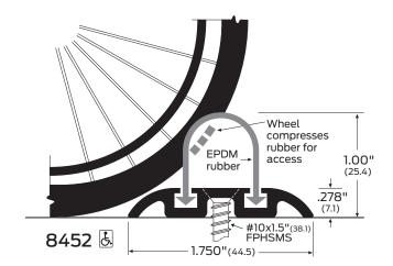
Press in the other edge of rubber into the second channel using your thumb or a screwdriver.
