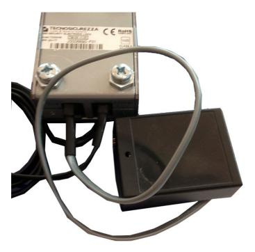
2) Connect the N42170/M magnetic Dallas key connection cable to the Dallas key reader or the T42146/J molex/jack connection cable as shown in the picture below.
