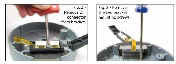
• Next use a slotted head or #1 Phillips head screw driver to remove the two bracket mounting screws (Fig. 3). Lift the bracket and thread the ZIF connector through the bracket cavity.
