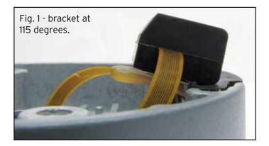
Prior to installing an X-O series lock, inspect the ZIF connector bracket. If the bracket is at 115 degrees, we recommend the following procedure.
