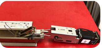
14. FLIP PUSH PAD OVER WITH KIT HOOKED IN & RE-INSTALL (2) PINS TO SECURE PUSH PAD TO BASERAIL. MAKE SURE OPENING ON THE BOTTOM OF THE MOTOR BRACKET LINES UP WITH SET SCREW IN BASERAIL.
