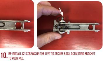
**9.** PLACE BACK ACTIVATING BRACKET BACK INTO THE PUSH PAD & LINE UP WITH EXISTING SCREW HOLES.
