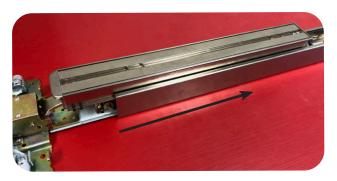
7 REMOVE (2) PINS SECURING PUSH PAD TO BASERAIL.
