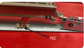
7. FLIP BASERAIL & PUSH PAD OVER TO SECURE MOTOR MOUNT WITH (2) SCREWS PROVIDED.
