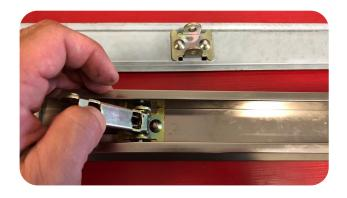
**5.** HOLDING ACTIVATING BRACKET IN PLACE, GRAB MOTOR KIT & HOOK ONTO THE PIN ON THE OUTSIDE OF THE ACTIVATING BRACKET. NEXT, ROTATE MOTOR KIT 180 DEGREES TO THE BACK OF THE PUSH PAD.
