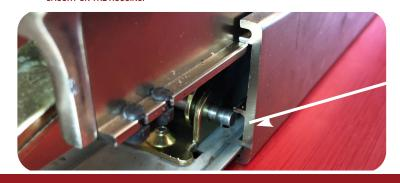
$16. \ {\small \hbox{SLIDE BASERAIL INTO HOUSING MAKING SURE THE BASERAIL SLIDES INTO THE}} \\ {\small \hbox{CORRECT CHANNEL}}.$
