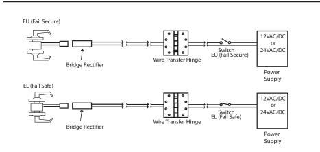
**STEP 4**: Connect the wires exiting the lock pocket to the Bridge Rectifier (included).
