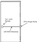
STEP 2: Run the wires from the ETH hinge through the 3/8" raceway starting at the ETH hinge & exiting into the lock pocket.
