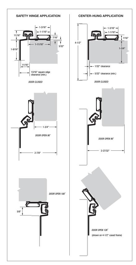
MATERIAL: Extruded 6063 T6 aluminum alloy with self-lubricating polyester thrust bearings.
