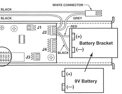
Battery plugs in place with polarity connected as shown
